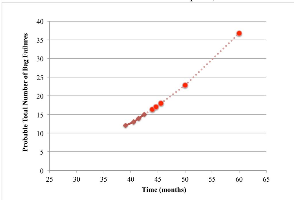
† Projected bag failures indicated by dotted line.
