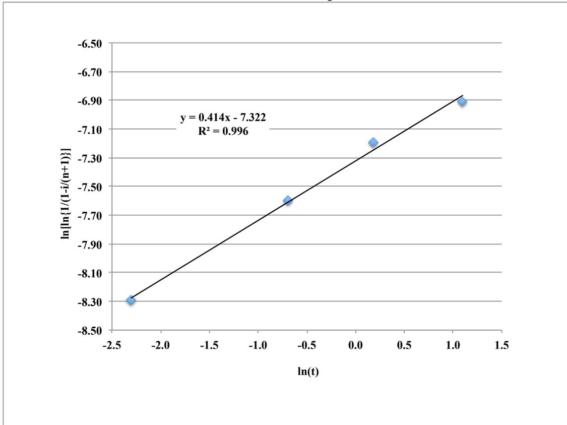
**Table 2. Summary Results of Weibull Coefficient Determination from Bag Failure Data Presented in Illustrative Example 2.**
