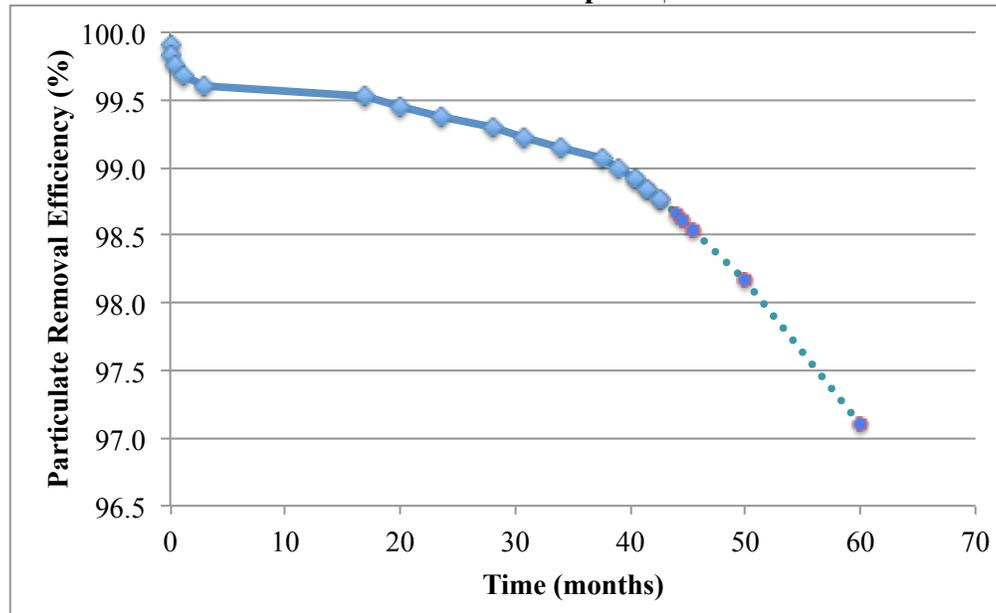
† Projected particulate removal efficiency results indicated by dotted line.
